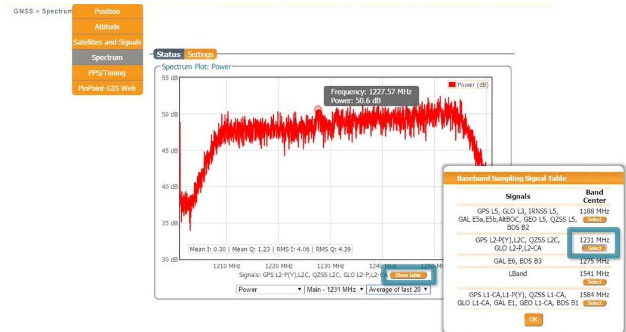
Figure 6-2: The RF spectrum of the L2 Band
